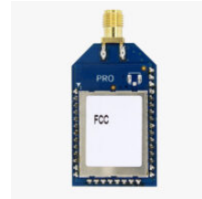
Plugins Radio module eXtra Long Range (XLR)
