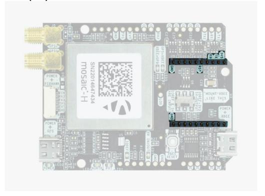
The simpleRTK3B Pro board has a High Power (HP) XBee socket. You can use this socket to connect any XBee compatible plugin. The following pins are available:
