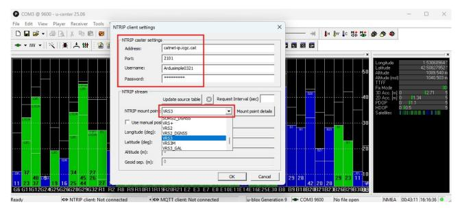
In a few minutes, you will see the Fix Mode change to FIXED or FLOAT. With valid FIXED you should see the 3D Acc.(accuracy) and 2D Acc.(accuracy) is centimeterlevel.
