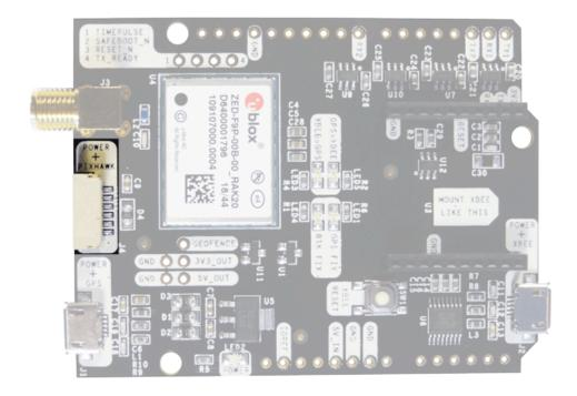
This connector is a standard JST GH that can be used to connect the simpleRTK2B to a Pixhawk autopilot. You can also use this connector to power the board.
