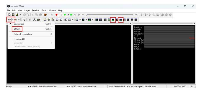
5. In the views toolbar, you can choose the data you want to visualize. We recommend to enable **GPS data** and **Satellite levels** to check the coordinates and signal strength.
