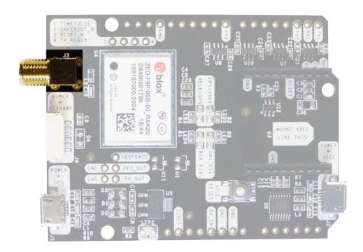
simpleRTK2B requires a good quality GPS/GNSS dual band antenna. The board is compatible with both active antennas supporting 3.3V supply and passive antennas. The maximum output current is 75mA @ 3.3V.
