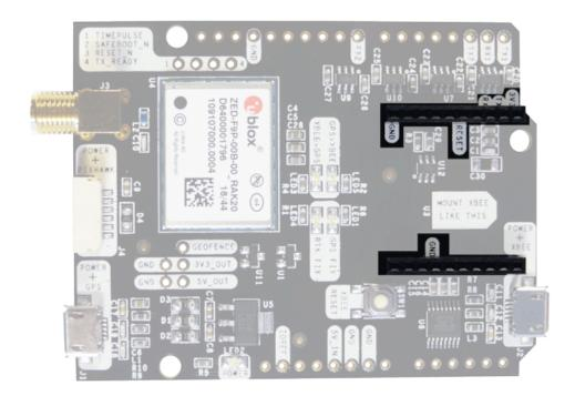
You can use this socket to connect an XBee compatible plugin. The following pins are available:
