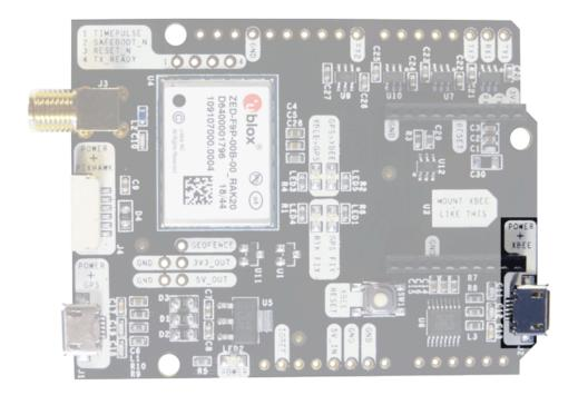
This micro-USB connector gives you access to the UART of the XBEE radio (if you mount one), via an FTDI USB-to-UART converter.
