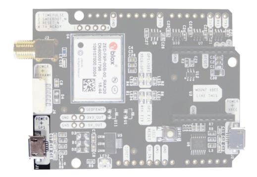
This micro-USB connector gives you access to the native USB from the ZED-F9P module. You can receive NMEA with the position, or have full access to the ZED-F9P using the ucenter tool: <a href="https://www.u-blox.com/en/product/u-center">https://www.u-blox.com/en/product/u-center</a>
