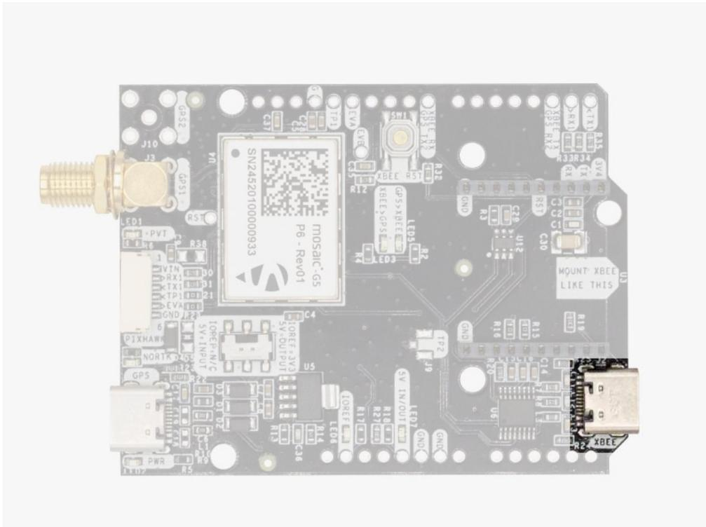
This USB-C connector gives you access to the UART of the XBEE radio (if you mount one), via an **FTDI USB-to-UART converter**.
