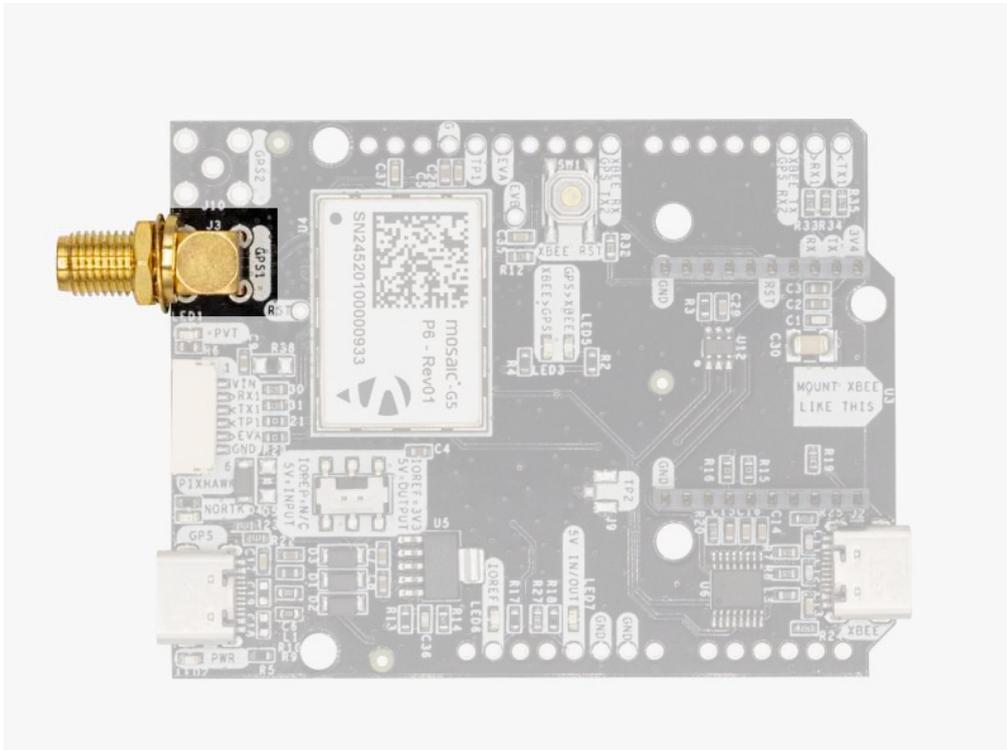
The simpleRTK 4 Pro does not include, but requires a high-quality **GPS/GNSS triple band (L1/L2/L5) antenna**. In order to get the best performance we recommend using our [Triple Band simpleANT3B series antenna](#).
