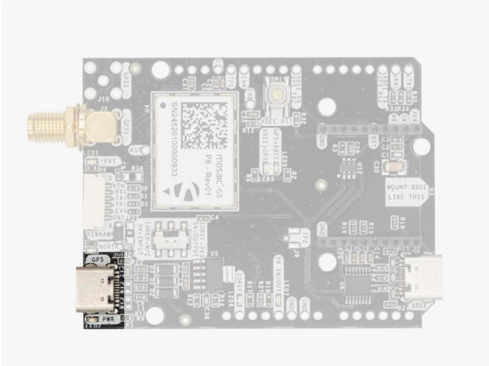
This USB-C connector gives you access to the native USB from the Mosaic module. When you connect to the PC for the first time, you will only see a new Hard Disk in your computer. Open it and install the Septentrio drivers.
