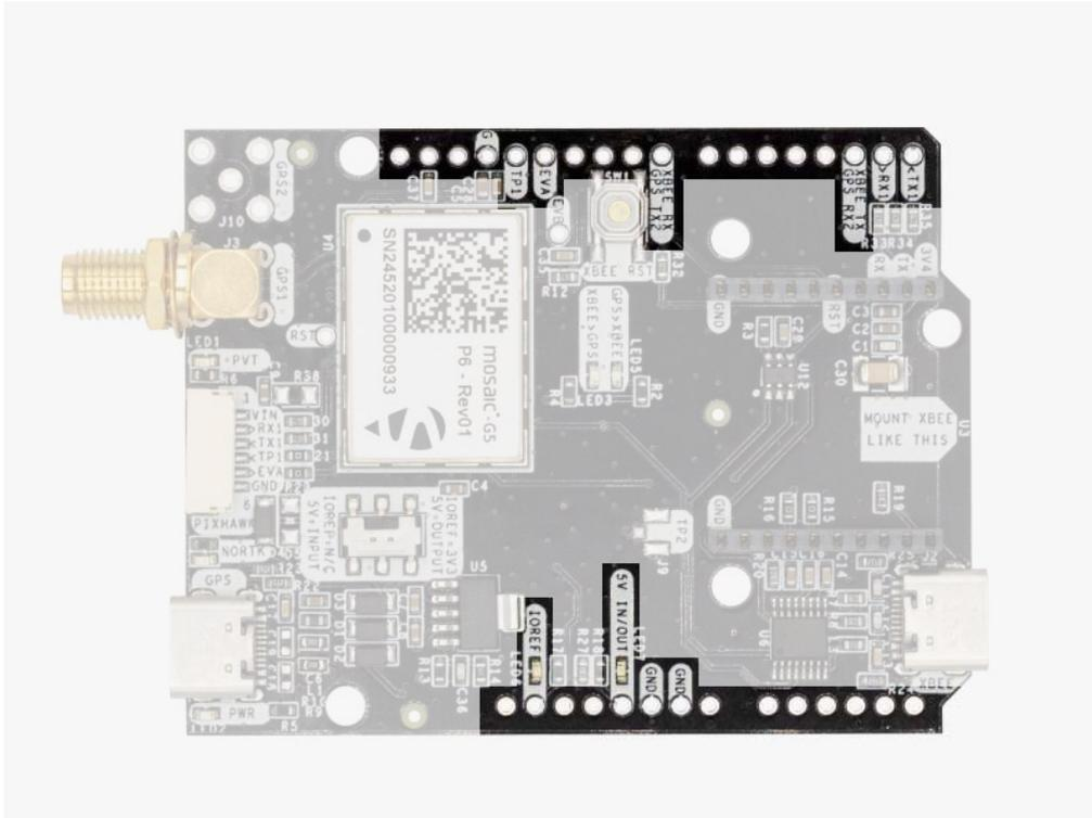
simpleRTK 4 Pro has optional rails to connect to other arduino UNO compatible devices.
