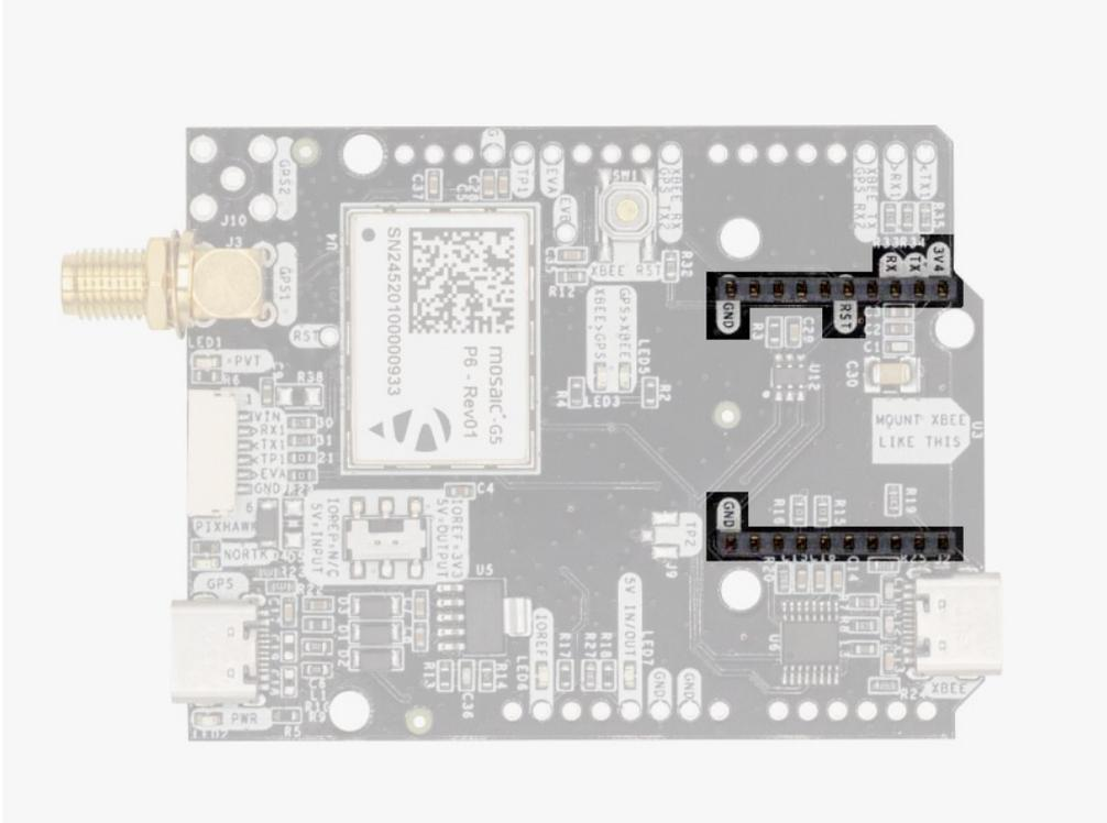
The simpleRTK 4 Pro has a High Power (HP) XBee socket. You can use this socket to connect an XBee compatible radio. The following pins are available:
