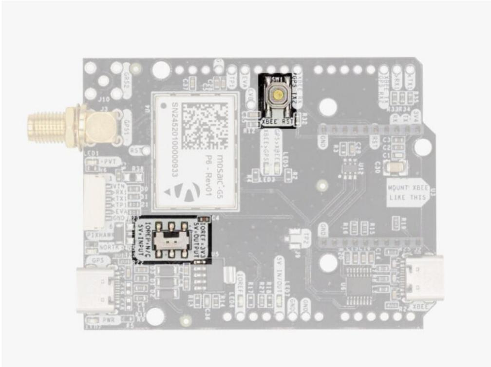
There's only one button: XBee Reset, and the good news is that you probably will not have to use it. This button is used to program the XBee radio if you want to update firmware, etc.
