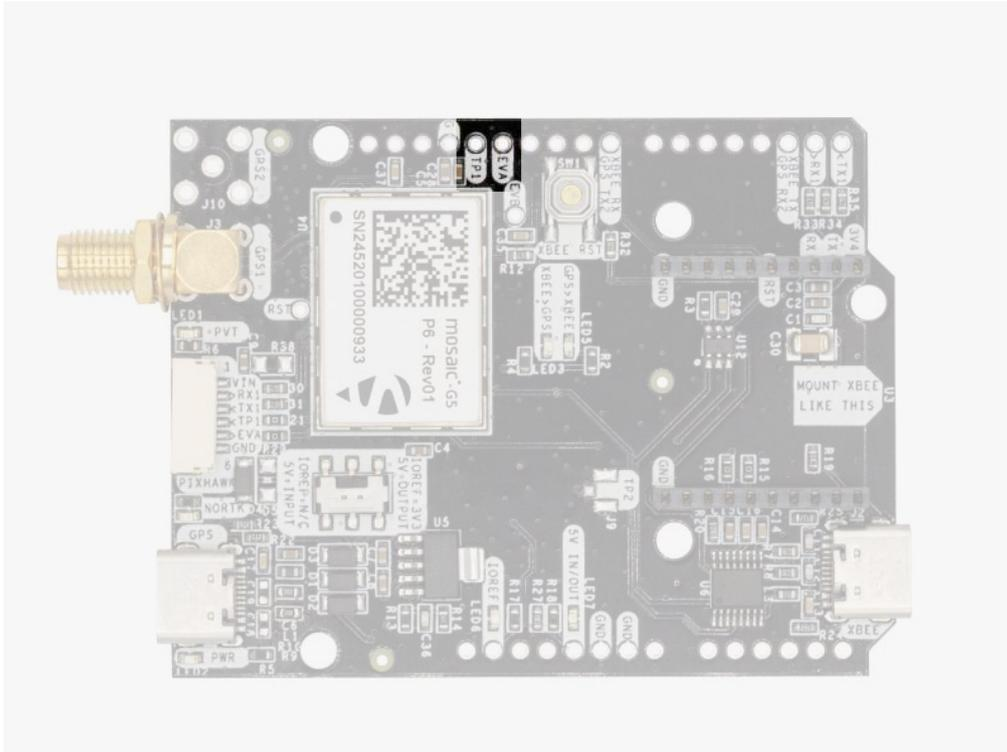
In addition to above, there's also a few additional pins available for the most advanced users. If you are going to use simpleRTK 4 Pro connected on top of an Arduino or Raspberry Pi and you don't use any of these pins, it's recommended to not connect the pins: you can cut the header in this pins to avoid the connection, and prevent unexpected behaviors.
