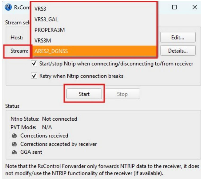
27. If the connection is successful, the **Status** field in the NTRIP Settings dialog should indicate that a connection has been established and that correction data is being received.
