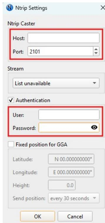
26. If the NTRIP account credentials were entered correctly, the **Stream** drop-down list will become active, and you can select your RTK correction **Mount Point**. Then, press **Start**.
