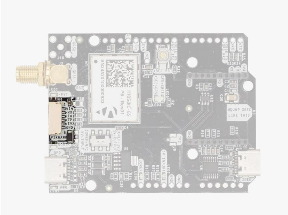
This connector is a standard **JST-GH** that can be used to connect the simpleRTK 4 Pro to a **Pixhawk autopilot**.
