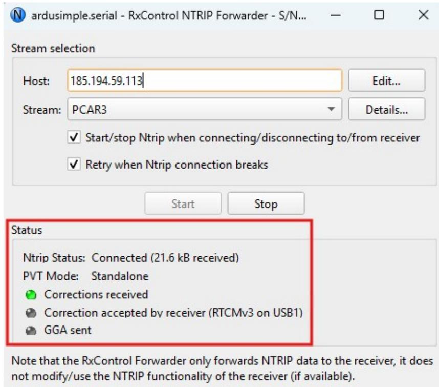
28. After a few minutes, the **PVT Mode** should change to **RTK Float** or **RTK Fixed**, indicating that your receiver has now achieved centimeter/millimeter-level accuracy.
