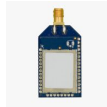
Plugins Radio module eXtra Long Range (XLR)
