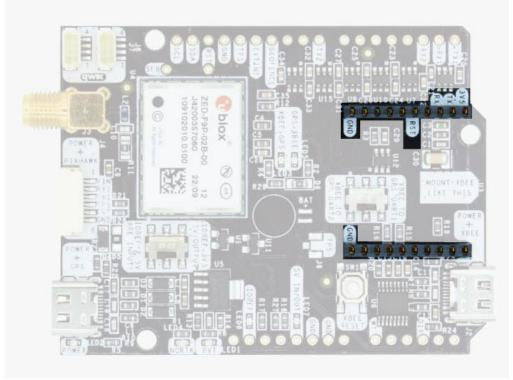
With simpleRTK2B V3 we introduce the new High Power (HP) XBee socket. You can use this socket to connect an XBee compatible radio. The following pins are available:
