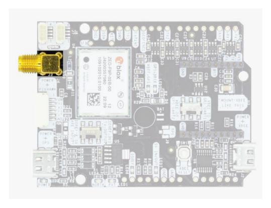
simpleRTK2B V3 requires a good quality GPS/GNSS dual band antenna.
