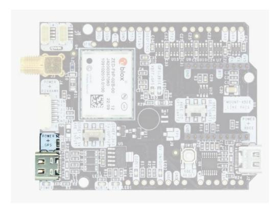
This USB-C connector gives you access to the native USB from the ZED-F9P module. You can receive NMEA with the position, or have full access to the ZED-F9P using the ucenter tool: <a href="https://www.u-blox.com/en/product/u-center">https://www.u-blox.com/en/product/u-center</a>
