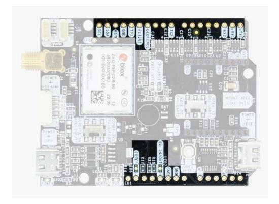
simpleRTK2B has optional rails to connect to other arduino UNO compatible devices.
