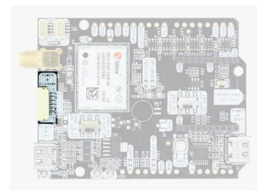
This connector is a standard JST GH that can be used to connect the simpleRTK2B V3 to a Pixhawk autopilot.
